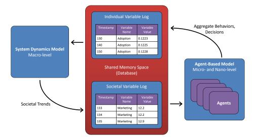
Fig. 5. Interaction between models using a shared memory space
